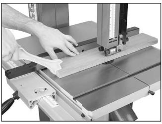
Figure 39. Ripping with a push stick.
